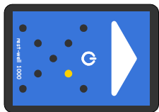
Figure 6: In this example the corner steady at the front right needs to be raised a little.
